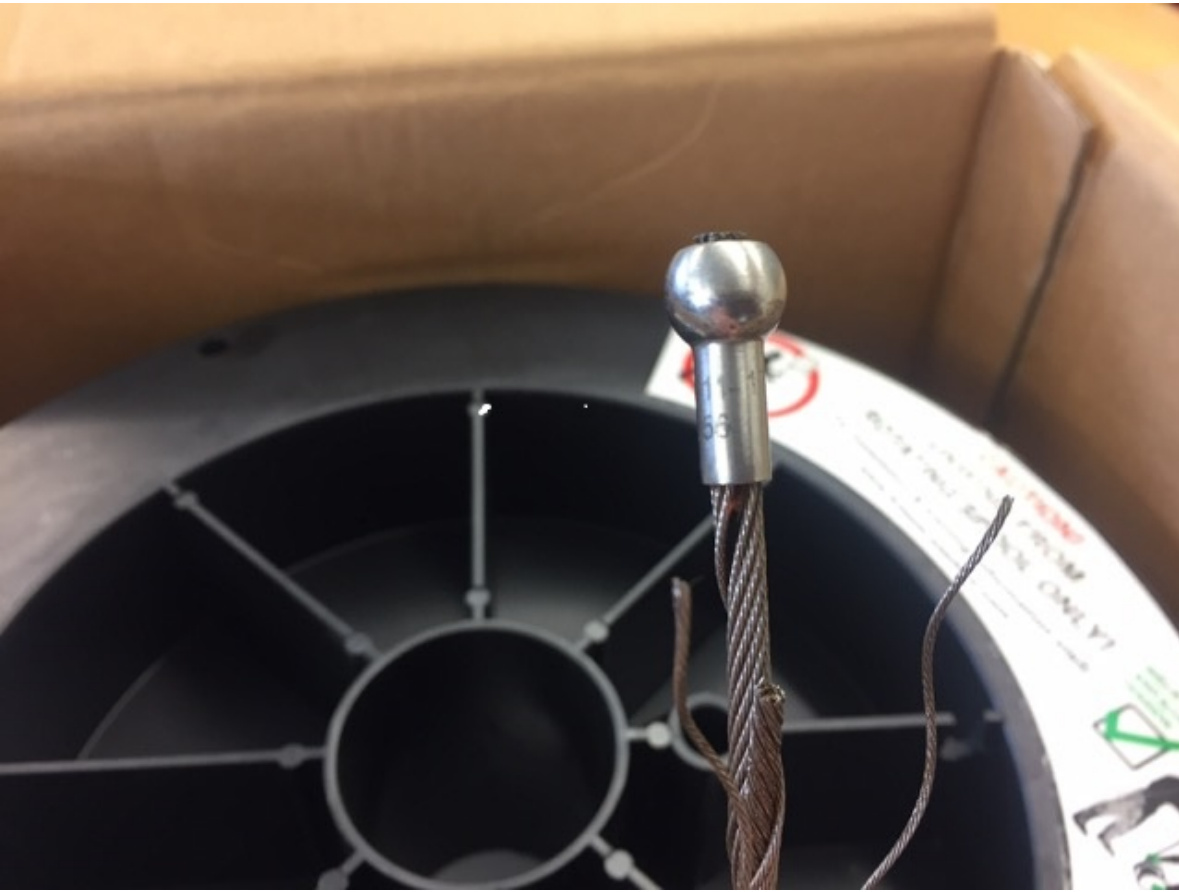
Inner wire and two outer strands found broken.
