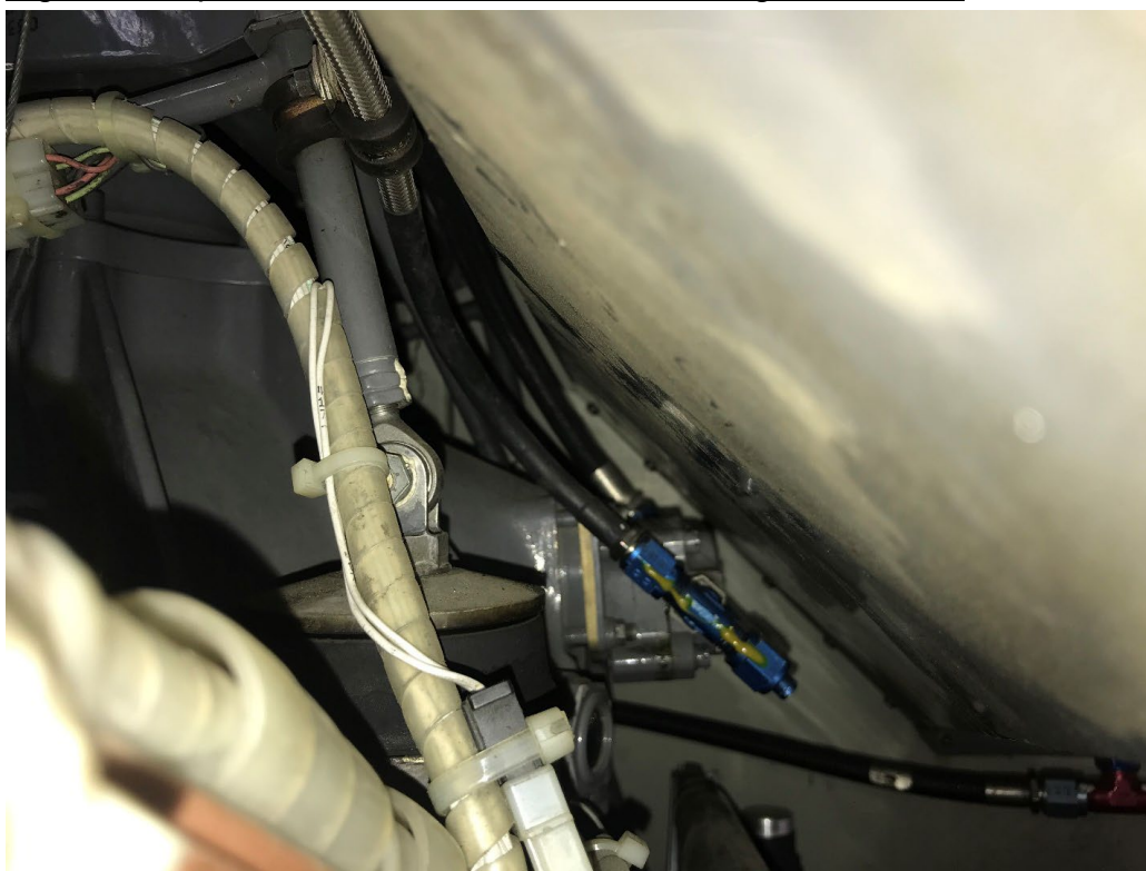
Fig 2. Example of correct orientation of the fittings and hoses
