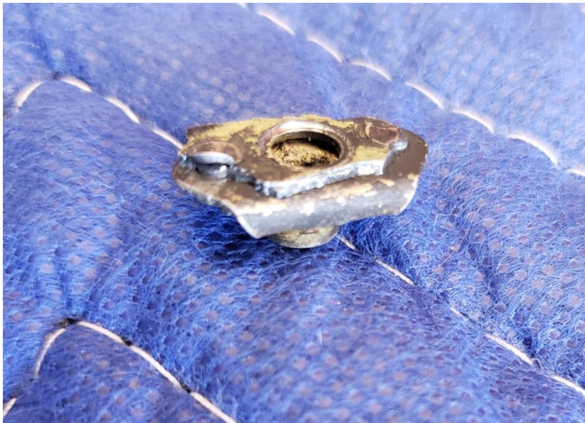
Picture 3 – Anchor nut with piece of rudder rib 6 still attached
