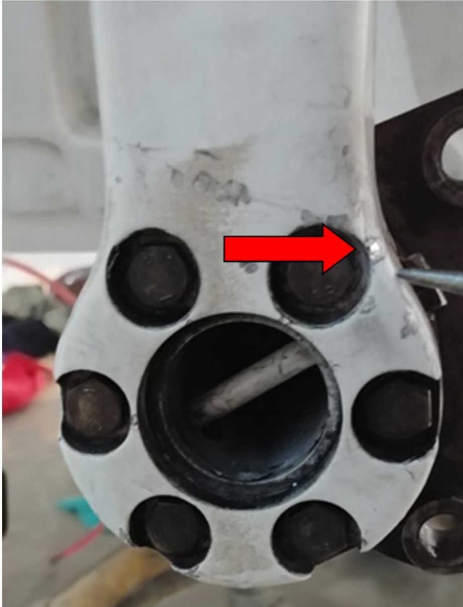
Figure 1 – Strut assembly fork – Crack location
