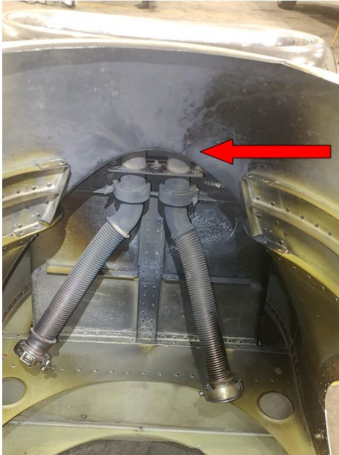
Picture 2 – Approximate location of weld failure
