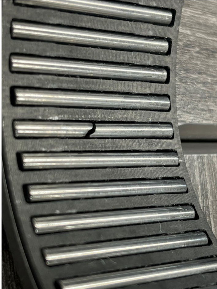
Fractured roller in bearing P/N 206-011-118-001
