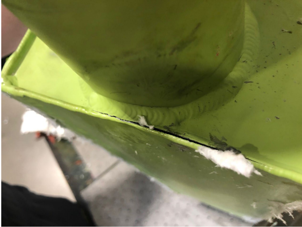
Picture 2 – Muffler outer wrapping removed, cracked at upper weld seam
