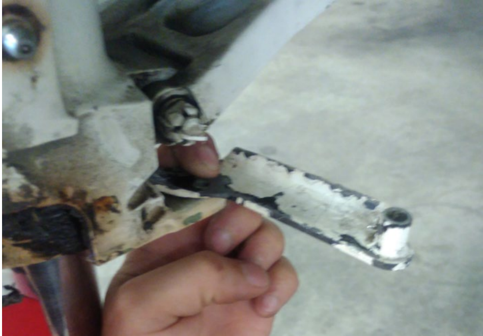
Figure 2 – Incorrect orientation of centering spring bracket
