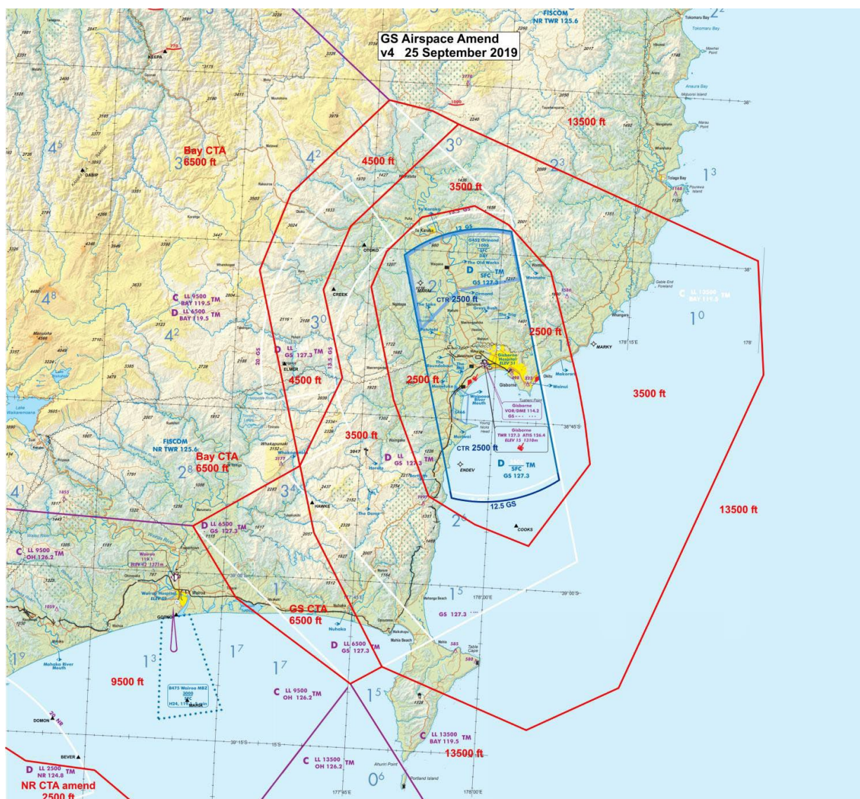
Diagram 1 DRAFT amended GS CTR and CTA version 4 Note minimal change to the GS CTR boundaries except that the upper limit is lowered to 2500 ft. White lines are the existing airspace boundaries to be deleted
