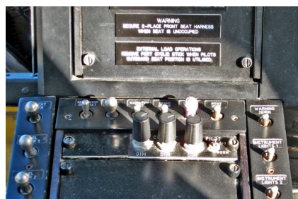
Dimmer controls on an AS350B2. Same helicopter type but different controls and position
