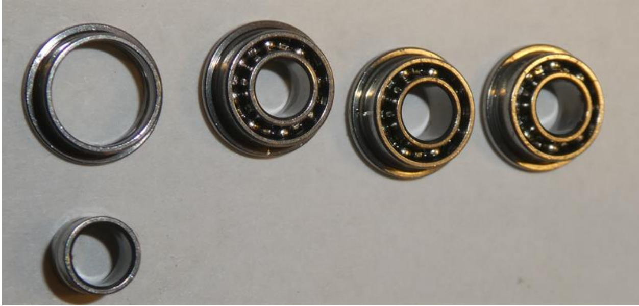
Figure 2 – Damaged and serviceable flyweight bearings
