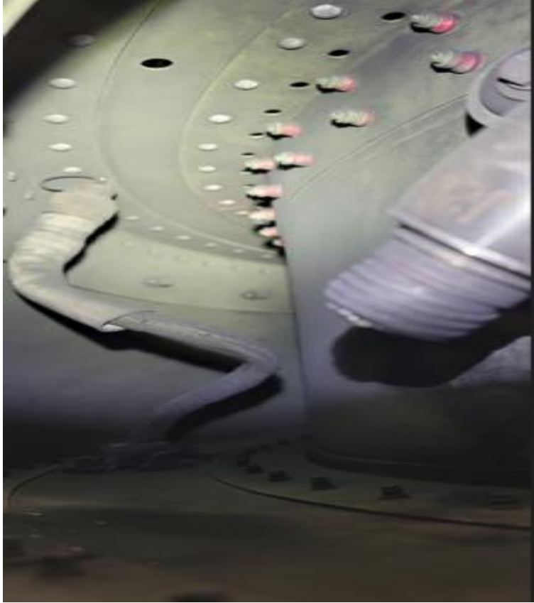
Picture 1 - Disconnected P20 electrical connector
