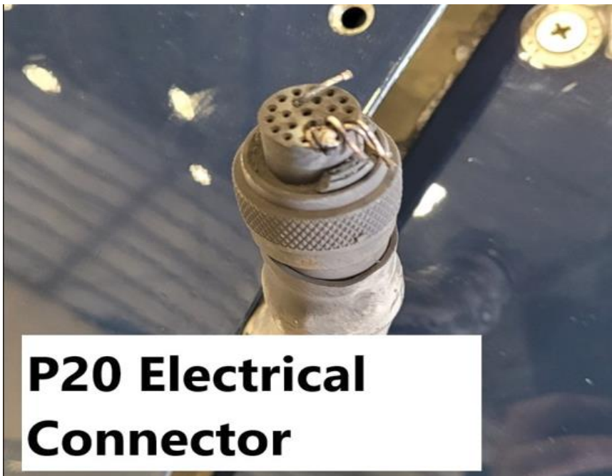
Picture 3 - Damaged P20 electrical connector
