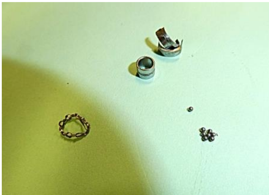
Figure 1 – Damaged flyweight bearing
