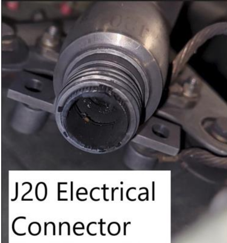
Picture 2 - Damaged J20 electrical connector
