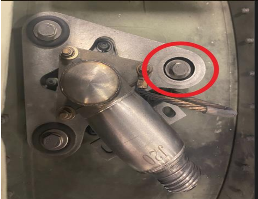
Picture 4 - Missing mounting grommet
