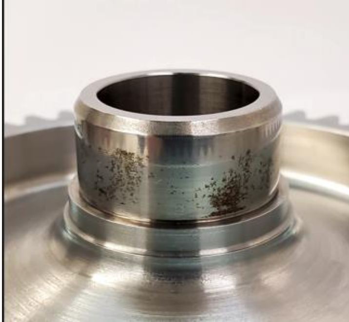
Picture 1 – Corroded gear shaft
