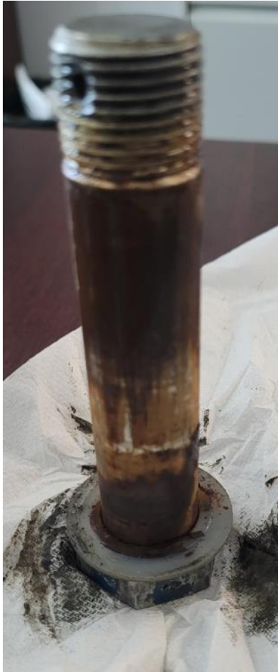
Figure 1 – Forward lower wing attachment bolt – Corrosion evident
