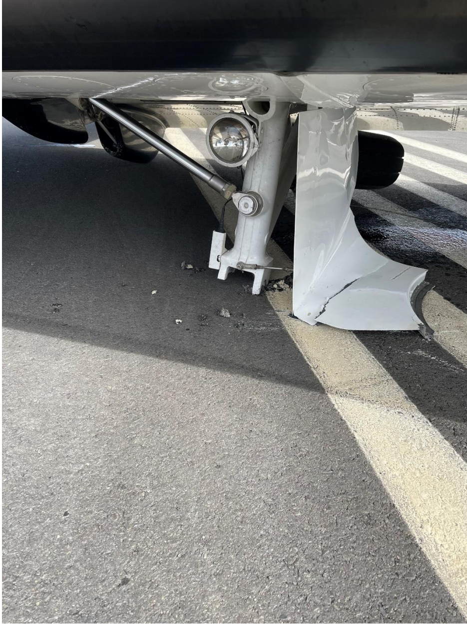
Picture 1 – Fractured gear impacting the runway
