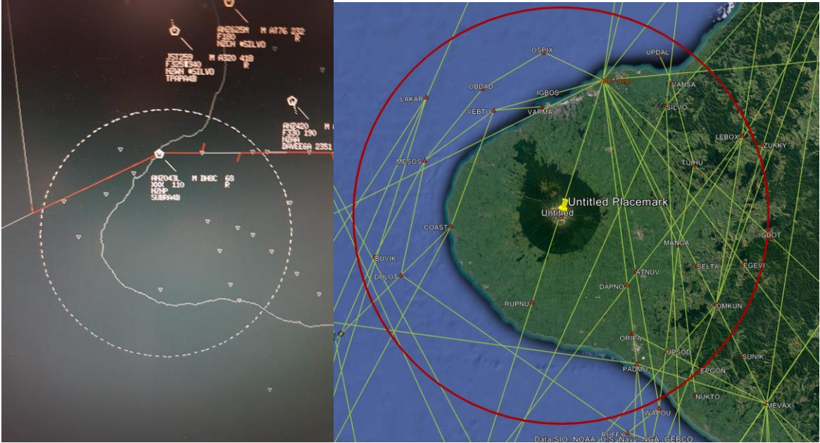
Figure 3: Overlay of VHZ area on Airways radar screen (left) and overlay of VHZ with published routes (right).
